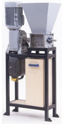
Gambar I.1 Mesin Pencacah Plastik ( Shredder Machine ) Sumber: ( www.preciousplastic.com )
