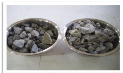
Fig. 1: Coarse aggregates, natural (left), recycled (right)
