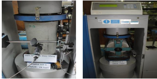
Fig. 4: Material test: Compression (left), Splitting (right)
