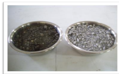
Fig. 2: fine aggregates, natural/sand (left), recycled (right)
