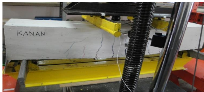
Fig. 6: RC-Beam under third point loading bending test
