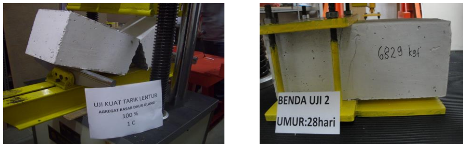
Fig. 5: Material test: Flexural (left), Shear (right)
