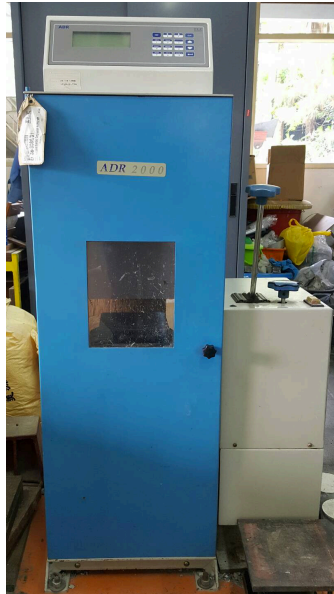
Gambar 1.1 Compression Testing Machine
