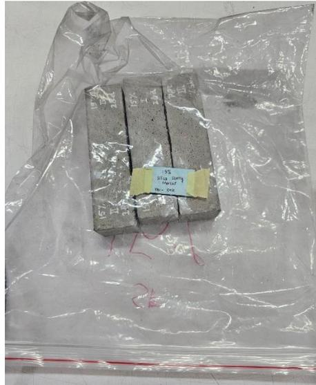
**Gambar 3.10** Metode *sealed curing*
