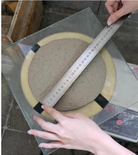
**Gambar 3.9** Pengukuran diameter pengujian *flowability*
