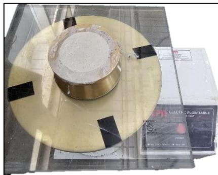
**Gambar 3.8** Uji *flowability* mortar
