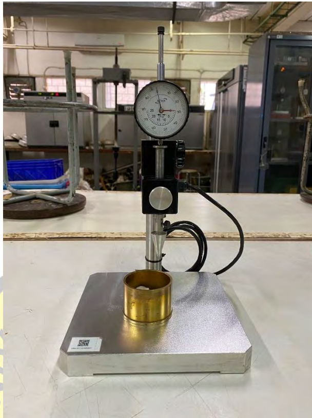
Gambar 1. 1 Fallcone Penetrometer Test
