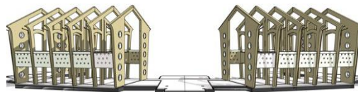
Fig. 10. The pentagonal shape and ventilation blocks as the most defining characteristic of Jengki -style architecture in BPH Building
