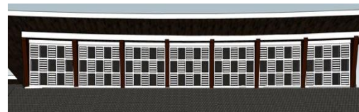
Fig. 14b. Closer view of ventilation blocks
